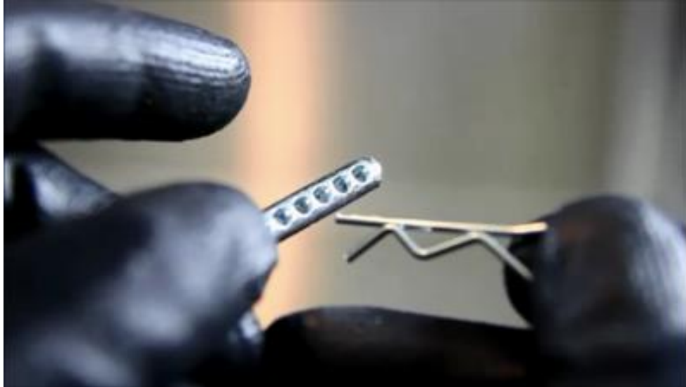
Picture 2. Always insert the straight side of the clip into the lock pin's hole.
